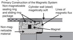
For this sensor principle it is not sufficient to simply mount the permanent magnet onto the piston. A magnetic system has to be constructed which conducts the magnetic flux of the permanent magnets directlt into the cylinder wall in order to achieve the strongest possible magnetization. For further details regarding the construction of magnetic systems, refer to the manual. A field trial is generally recommended before practical operation!
